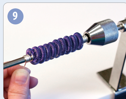
Start and finish the bead with a few extra coils.
