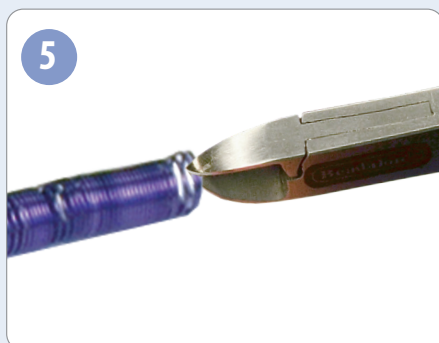
Remove Coil from Rod. Flush-cut the inside of the coil.
