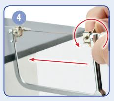
Apply pressure from the end of the saw so that the blade is guided into the other fixture. Tighten the wing nut.
