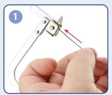
Loosen the wing nuts on the saw and insert the blade with the teeth pointing out and down.
