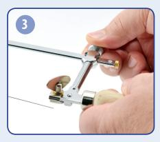
Adjust the saw arm to fit the blade, then carefully position the other end of the blade into the saw frame fixture.
