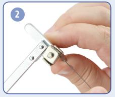
Slip one end of the blade into the fixture and tighten the wing nut.
