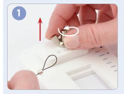
Unscrew the wing nut at the upper part of the Tying Station. Make a loop with your cord and tie or crimp it.
