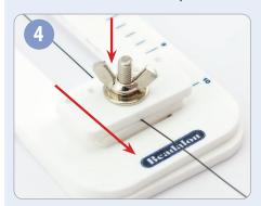
Loosen wing nut at the base of the Tying Station. Slide cord between acrylic plates. Tighten as needed to keep cord secure.
