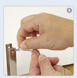
Pull all the wires taught and attach to a sturdy object (door knob, nail, or screw eye attached to a workbench or wall).
