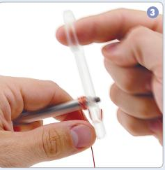
Hold wire across the mandrel with one hand, then insert a finger from your other hand into the large hole in the handle and turn clockwise, make as many revolutions as desired.
