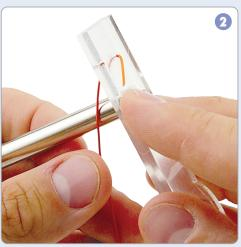
Insert wire into the small hole in the handle, fold the wire down to secure.
