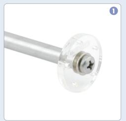
Assemble the wire twister by first removing the screw in the end of the wire twister. Then, place up to 5 wires into the holes of the disc, any diameter desired up to 18 gauge (1.02mm) the acrylic disc in between the two washers, then insert the screw and tighten.
