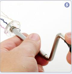
Turn the crank while holding the shaft, continue turning until the desired twist is achieved, turning until breakage assures the most hardening and tightest twist.
